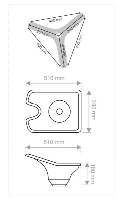
Mobile wash station, stand with cast iron base, grey powder-coated, height adjustable: 80-110 cm, "standard edition" with drain hose and hook, length 200 cm, hose inner diameter ø 22.2 mm
